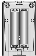
■ (Place the batteries with their terminals corresponding to the (+) and (-) indications in the battery compartment.)
